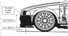
no point may any part of inflexible material for bodyshell mounting protrude from the body more than 10mm. If an opening is created through the foam bumper for cooling air, the combined thickness of the foam (above and below the cooling hole/slot) must still be a minimum of 40mm in height.
